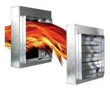
**OPERATION:** Fire dampers (Figure 1) are operated by a fusible device, typically a melting link. They are designed and tested under UL Standard 555: Standard for Safety for Fire Dampers, to maintain the integrity of the fire-rated separation. Fire dampers are equipped with a fusible link (rated for 165°F up to 286°F), which holds the blades open until it the link melts. Upon reaching the melting point, the blades then close and stop the flame from moving into an adjoining compartment.
